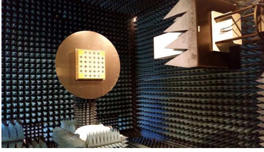
Fig. 3. 40-element PAF in nearfield-measurement range.
