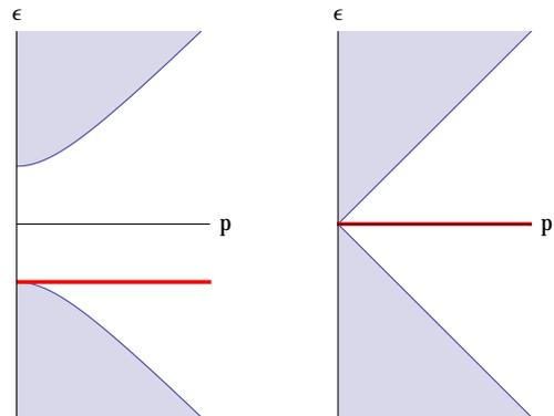
FIG. 1. The obtained dispersions (47) and (48). Left panel is for  $m \neq 0$ , while Right panel is for  $m = 0$ . The red lines are for the edge state (48) which is a flat band, and touches the tip of the bulk dispersion cone.
