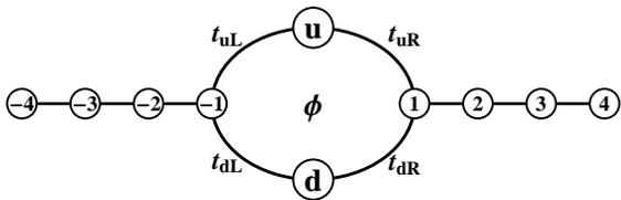
FIG. 1. Schematic setup of the Aharonov-Bohm ring system discussed in this paper.  $u$  and  $d$  are the two QDs embedded in the arms of the ring. The leads coupled to the ring are represented by two one-dimensional tight binding chains.  $\phi$  is the magnetic flux threading through the ring.
