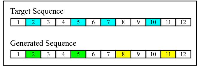
Fig. 2. Example of target sequence matching in discrete time, where the generated sequence is constrained by a charging time of  $n_{\min} = 3$  slots. Slots are labeled chronologically and colored when there is a spike at the start of the slot. The target sequence has 4 pulses (shown in blue). The generated sequence can match the first 2 pulses (green), but the final 2 pulses (yellow) each have a delay of one slot.
