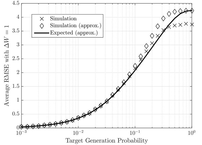
Fig. 3. Average RMSE  $\bar{d}(\vec{u}, \vec{v})$  as a function of the target firing probability  $p_T$  in each time slot. The expected analytical curve is evaluated from (11). The actual observed distortion is calculated using (8), and the approximate observed distortion is calculated using (9).
