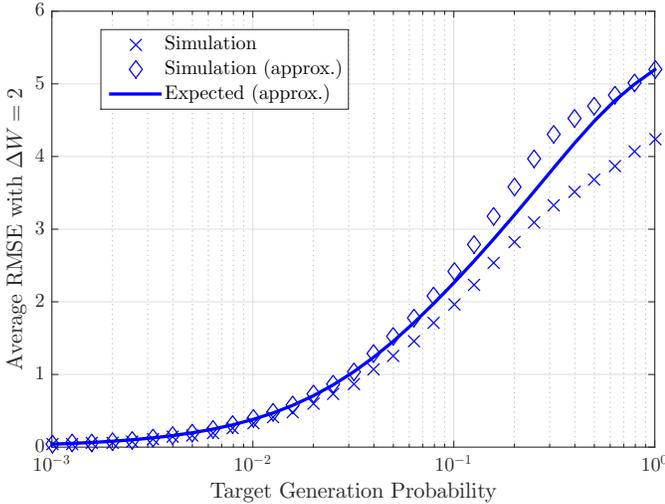
Fig. 5. Average RMSE  $\bar{d}(\vec{u}, \vec{v})$  as a function of the target firing probability  $p_T$  in each time slot. The metric kernel has length  $\Delta W = 2$  and coefficients  $\{h_0, h_1\} = \{\sqrt{0.5}, \sqrt{0.5}\}$ . The expected analytical curve is evaluated from (15). The actual observed distortion is calculated using (12), and the approximate observed distortion is calculated using (13).
