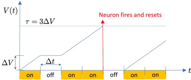
Fig. 1. Illustration of the neuron model with integrate-and-fire. In this example,  $n_{\min} = 3$ , i.e., spikes must be separated by at least  $3\Delta t$ . In each interval when the light source is on, the voltage increases by  $\Delta V$ . Once the threshold  $\tau = 3\Delta V$  is reached, the neuron fires and resets to  $V(t) = 0$ .
