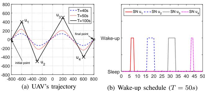
Fig. 1. The UAV's trajectory and SNs' wake-up schedule.
