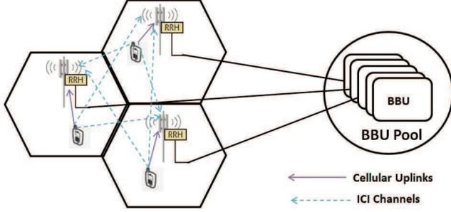
Fig. 1. System model of C-RAN with ICI
