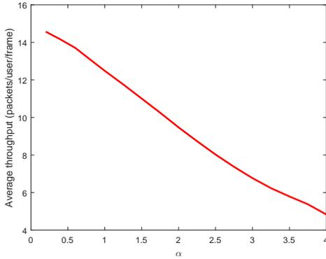
Fig. 5. Throughput vs. power control parameter  $\alpha$
