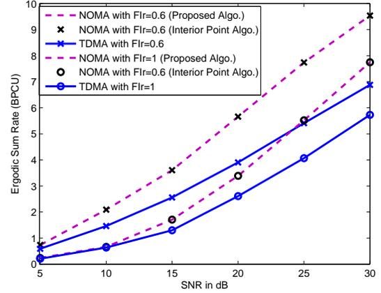
Fig. 5. Ergodic sum rate vs SNR in dB, where  $K = 5$ ,  $\text{SNR} = 20$  dB,  $\text{FIR} = 0.6, 1$ .
