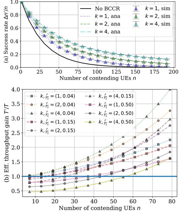
Fig. 3: Above: (a) UE success ratio  $\Delta n'/n$ ; Below: (b) Effective throughput gain  $T'/T$  vs. number of contending (non-barred) UEs in a PRACH slot  $n$ .  $k \in \{1, 2, 4\}$  CRSSs;  $M = 30$ ; 95 % confidence intervals.
