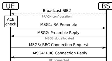
Fig. 1: Standard protocol for LTE Random Access Procedure.
