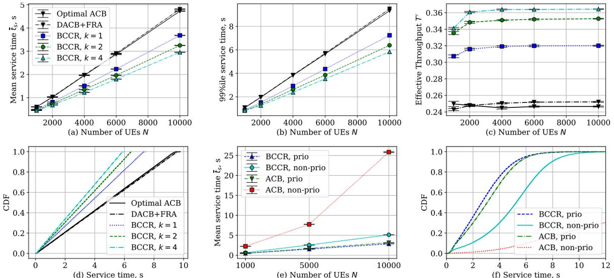
Fig. 4: Randomized priorities: (a) Mean and (b) 99%ile of the service time; (c) effective throughput  $T$  vs. number of UEs  $N$ ; (d) Service time CDF for  $N = 10000$ . Two-class prioritization: (e) mean service time  $\bar{t}_s$  vs. number of UEs  $N$ ; (f) Service time CDF for  $N = 10000$ ;  $T_A = 1$  s,  $\alpha = 3$ ,  $\beta = 4$ ;  $k \in \{1, 2, 4\}$  CRSs; D-ACB with FRA [7];  $M = 30$ ; 95 % conf. int.
