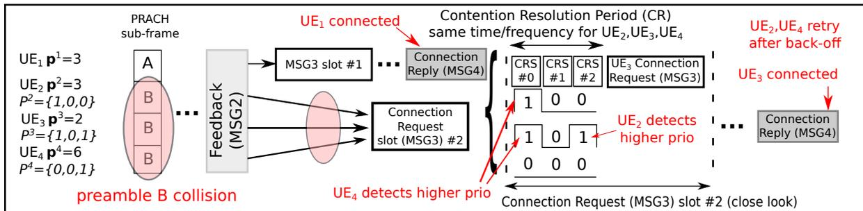
Fig. 2: Exemplary operation of RA procedure with Binary Countdown Contention Resolution.
