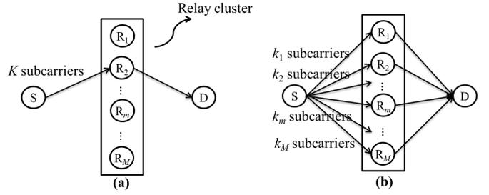
Fig. 1. Illustration of (a) bulk, (b) per-subcarrier relay selection schemes for single source, single destination and  $M$  clustered relays with  $K$  subcarriers. Note,  $K = \sum_{m=1}^M k_m$  for  $k_m \in \mathbb{N}, \forall 1 \leq m \leq M$ .
