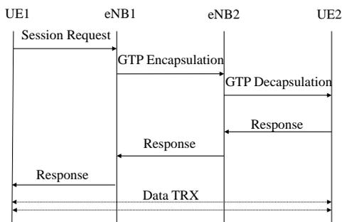
Fig. 3. Information flows between mobile users and the base stations.
