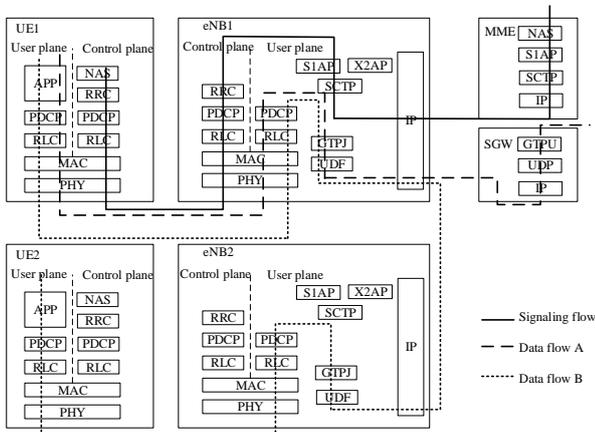
Fig. 2. A novel protocol for local breakout.
