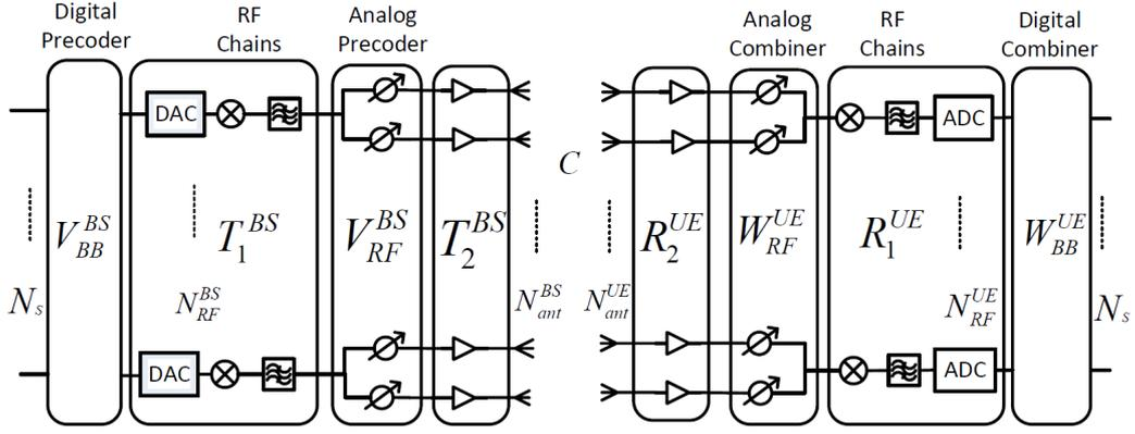
Fig. 3: Hybrid beamforming system where a BS (left) is transmitting  $N_s$  data schemes in the DL to a UE (right). The switches in the BS are connected to the transmit path whereas those in the UE are connected to the receive path.
