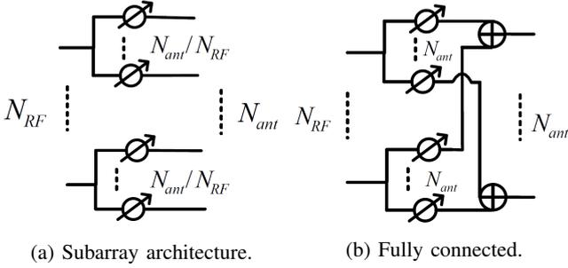
Fig. 2: Two types of analog beamforming structure.
