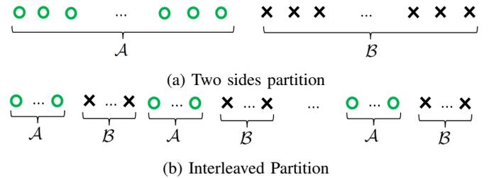
Fig. 7: (a) ‘‘two sides partition’’ where group  $\mathcal{A}$  and  $\mathcal{B}$  contain 32 antennas on the left and right sides of the linear antenna array, respectively; (b) ‘‘interleaved partition’’ where every 8 antennas are assigned to group  $\mathcal{A}$  and  $\mathcal{B}$ , alternatively.
