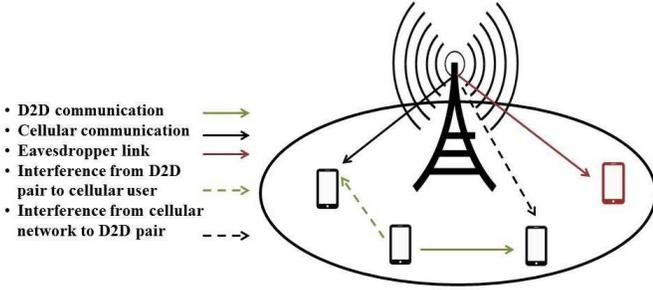
Fig. 1. A D2D communication underlaying an existing cellular network.
