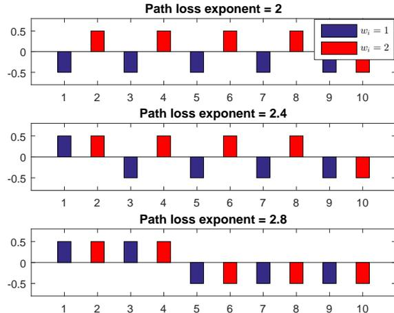
Fig. 4: Change of optimal computing modes of a heterogeneous case, where  $w_i = 1$  if  $i$  is an odd number and  $w_i = 2$  otherwise. The three figures show the performance under path loss exponent  $d_e = \{2, 2.4, 2.8\}$ , respectively.
