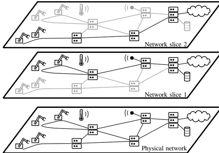
Fig. 1: Illustration of slicing a physical network into two logical sub-networks. Network slice 1 offers URLLC to an edge cache and the cloud, while network slice 2 provides an eMBB service to the Internet.
