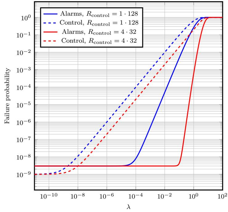
Fig. 5: End-to-end failure rate of control and sensor alarm traffic in the network slicing scheme based on overwriting for various alarm arrival rates.
