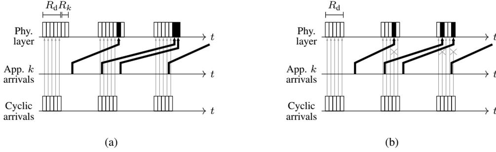
Fig. 2: Two methods of cyclic resource multiplexing: a) multiplexing of reserved resources between gateway arrivals; b) multiplexing by overwriting random cyclic traffic.
