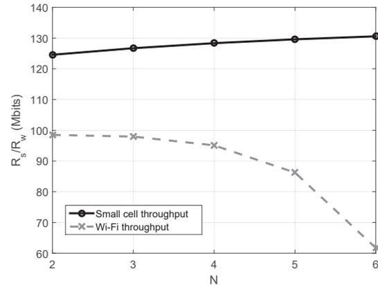
Fig. 3. Small cell and Wi-Fi throughput v.s. spatial DoF allocation
