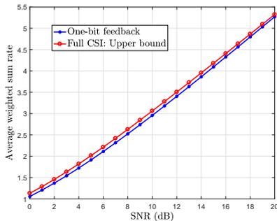
Fig. 2. Comparing the average weighted rate of our proposed one-bit feedback scheme with the full-CSI case (upper bound performance).
