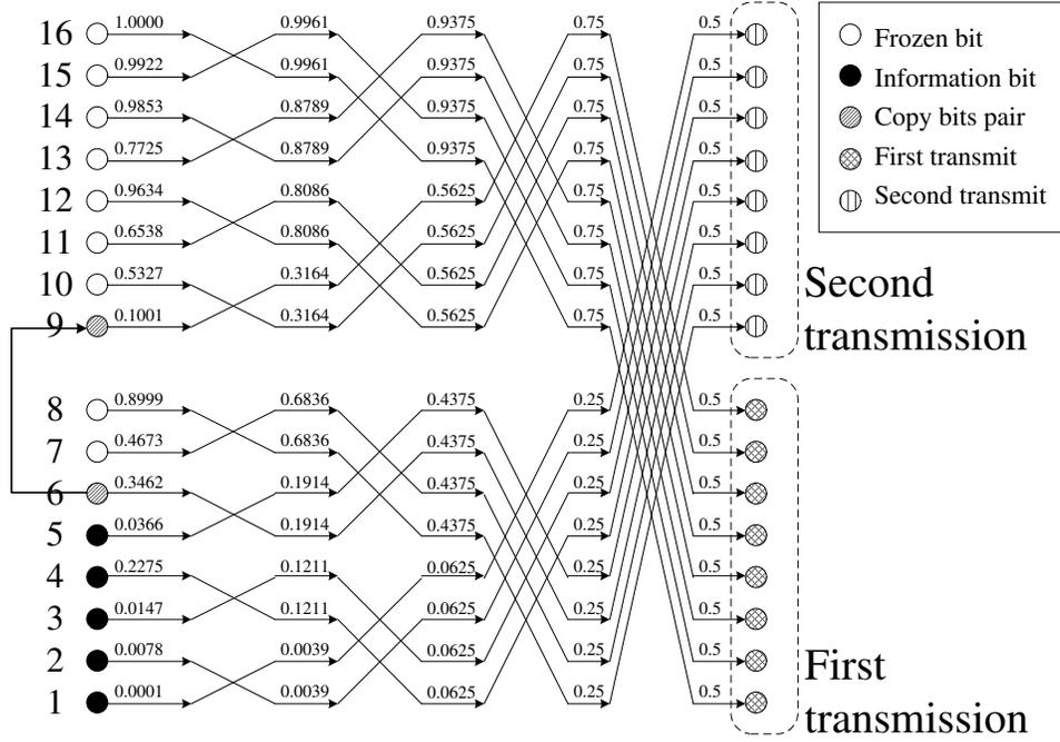
Fig. 2: An Extending Example from a (8, 6) polar code to a (16, 6) polar code
