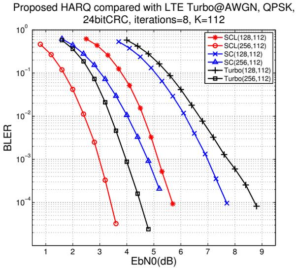
Fig. 6: Comparison between proposed algorithm and LTE Turbo code
