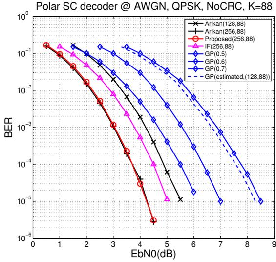
Fig. 5: The BER comparison between different HARQ algorithm with  $k=88$
