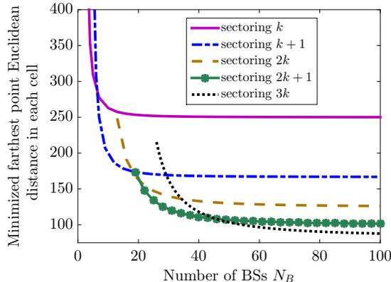
Fig. 3: Variation of minimized farthest point Euclidean distance with  $N_B$  in each cell for different type of sectoring.
