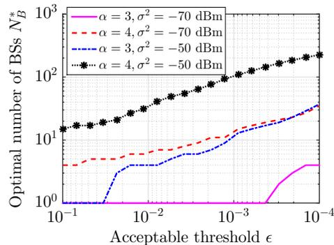
Fig. 9: Variation of optimal number of BSs with threshold  $\epsilon$  for different values of  $\alpha$  and  $\sigma^2$ .
