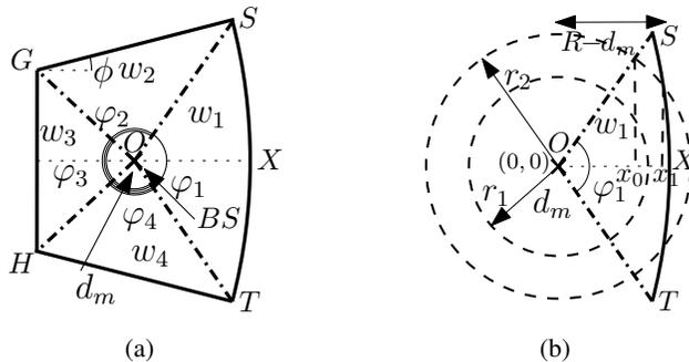
Fig. A.1: (a) Division of the  $m^{\text{th}}$  cell in four disjoint sub-fields  $\{w_j\}; j \in \{1, 2, 3, 4\}$ , (b) computation of distance distribution of an UE from location  $d_m$  of the BS over the sub-field  $w_1$ .
