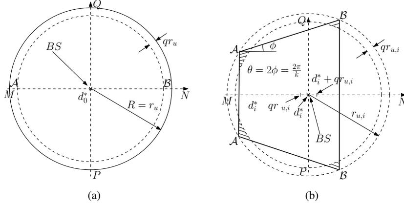
Fig. 4: Actual optimal location of a BS (a) in a circular field, (b) in an  $i^{\text{th}}$  cell for a given value of  $N_U$ .
