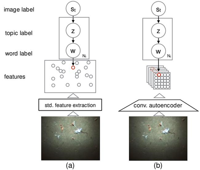
Fig. 1. Two scene modeling techniques evaluated in this paper. Here  $s_t$  is the image label, and  $z$  is the topic label of a visual word  $w$  in the input image. (a) A baseline spatiotemporal topic model using standard computer vision features as input. (b) The proposed spatio-temporal topic model using convolutional autoencoder-based features.
