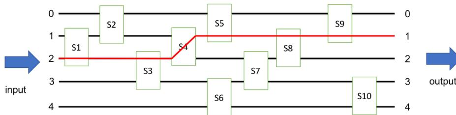
Figure 2 Modulo-5 RNS Adder with example  $2+4 = |6|_5 = 1$
