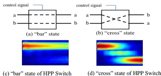
Figure 1 Two States of a  $2 \times 2$  Switch. (a) and (b): the conceptual schematic of two states in a  $2 \times 2$  switch. (c) and (d): the top view of the FDTD simulation results of two states in our  $2 \times 2$  Hybrid Photonic-Plasmonic switch with two silicon waveguides (up and down) as buses and a switching island covered by indium tin oxide in between to achieve signal switching. [9]
