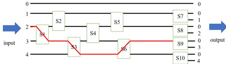
Figure 4 Modulo-5 RNS Adder with example  $2 \times 4 = |8|_5 = 3$
