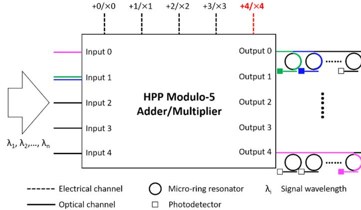
Figure 5 Schematic of WDM Modulo-5 RNS Computation Unit.
