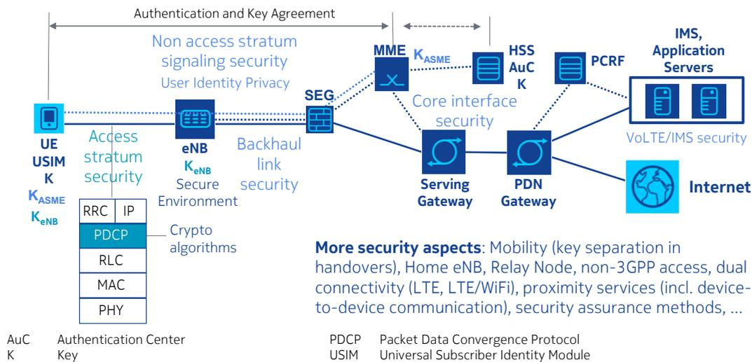
FIGURE 1. Security Architecture of 3GPP LTE / EPS [11]
