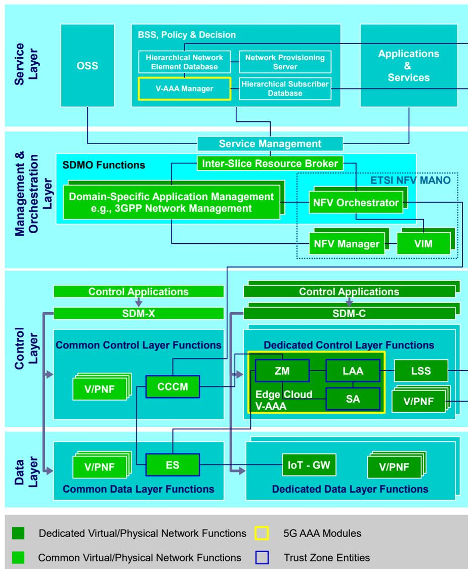
**FIGURE 2.** The 5G AAA framework enhanced with Trust Zone in the 5G PPP architecture. The terms OSS, VIM, SDM-X, SDMO and SDM-C stand for operations support system, virtual infrastructure manager, software-defined mobile network (SDM) controller, SDM orchestrator and SDM coordinator, respectively. V/PNF denote virtual/physical network functions.
