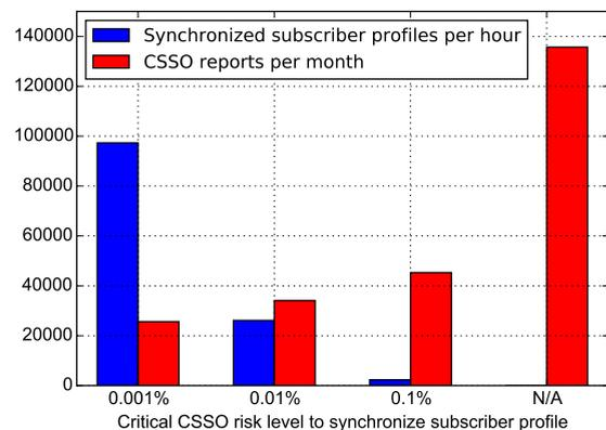
**FIGURE 7.** The performance of TZ under different specifications of decision threshold. Note that N/A stands for no TZ deployment, which is the baseline of LTE systems.
