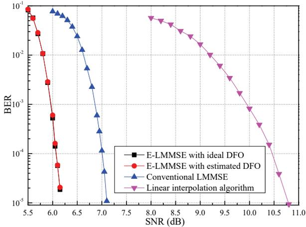
Fig. 4. BER of several channel estimation methods at the 3 dB power-difference position.
