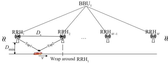
Fig. 1. HSR two-tap channel model.
