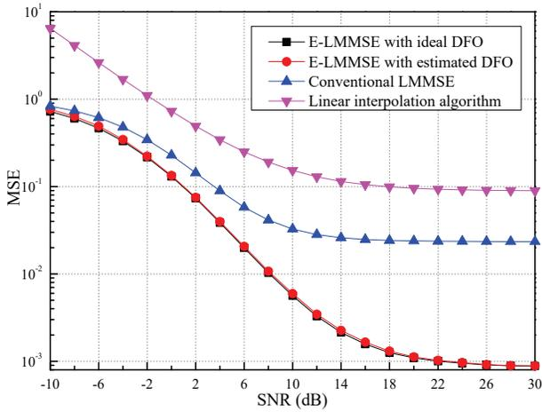
Fig. 3. MSE of several channel estimation methods at the 3 dB power-difference position.
