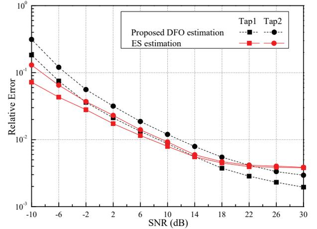
Fig. 2. Relative error of two DFO estimation algorithms at the 3 dB power-difference position.
