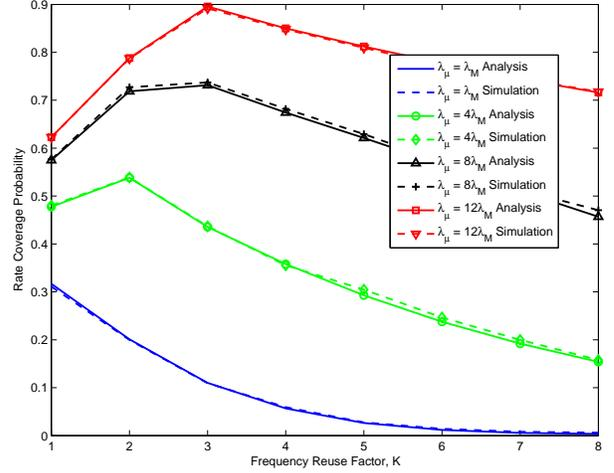
Fig. 9. Rate coverage probability with different micro density-to-macro density ratios  $\lambda_\mu/\lambda_M$ .
