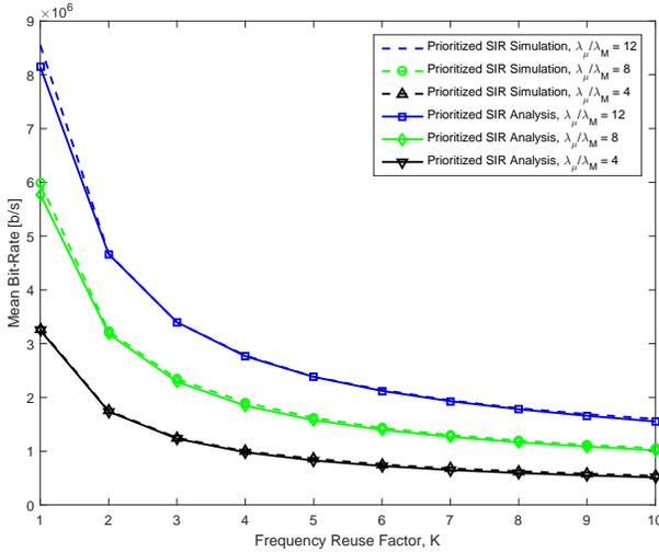
Fig. 11. Mean UE bit-rate rate as a function of the frequency reuse  $K$ .
