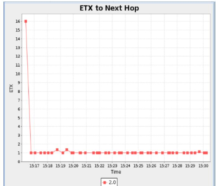
Fig 6: expected number of transmissions required to send the data to the data collector node
