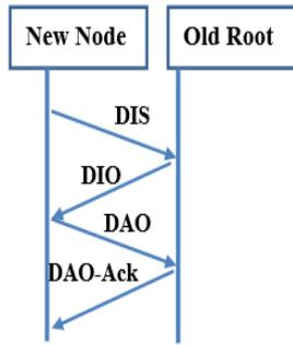
Fig 3: Flow diagram of control messages of RPL protocol
