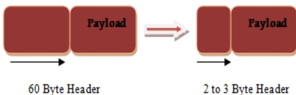
Figure 2 IP Header Compression from 40 bytes to 2-4 bytes [5].
