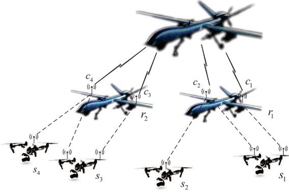
Fig. 1. A multi-channel and multi-radio UAV relay network.
