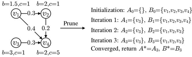
Fig. 2. An example of iterative pruning under the Independent Cascade diffusion model. Each node is associated with a benefit weight  $b$  and a cost weight  $c$ . Each edge has a propagation probability  $p$ .
