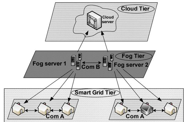
Fig. 5 Hierarchical communication structure of the Fog computing.
