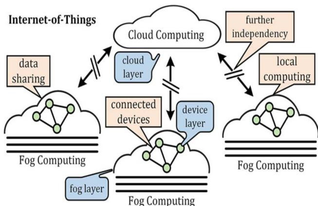
Fig. 8 Implementing Fog computing as an intermediary layer to cloud computing in Internet-of-Things (IoT) platform.
