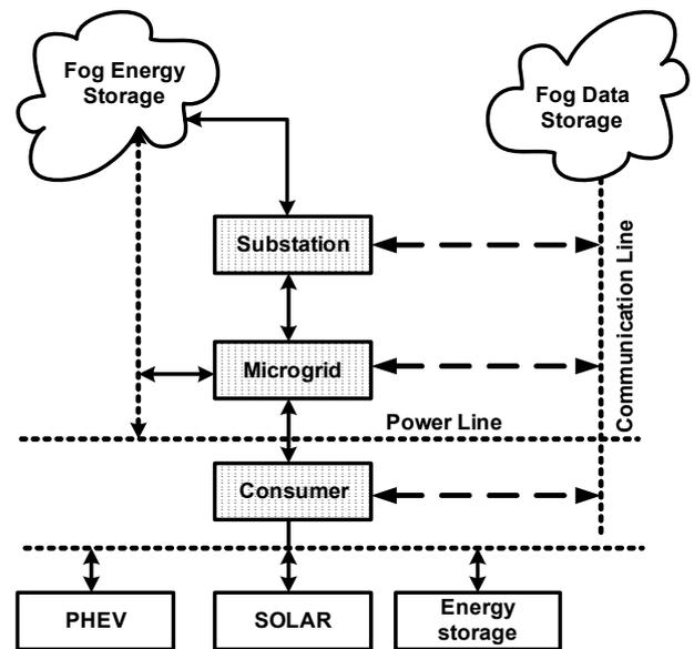
Fig. 7 Microgrid concept using Fog computing.
