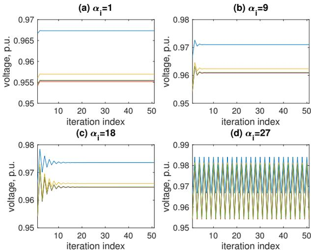
Fig. 6. Evolution of voltage of the dynamical system  $\mathcal{D}_1$  with different slopes of the piecewise linear control function: Voltage does not converge when the (absolute) slope of the control function become too large (when  $\alpha_i > 26$  in this example).
