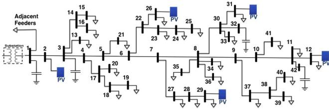
Fig. 4. Circuit diagram for SCE distribution system.
