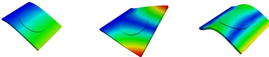
Figure 5: Contour plot of the first three eigenforms of plate with circular patch actor
