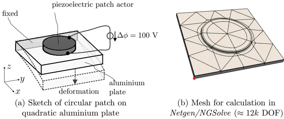
Figure 3: Sketch and mesh for circular piezoelectric patch actor
