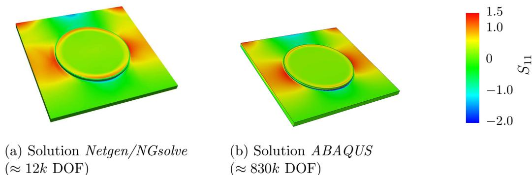
Figure 4: Contour plot of stress  $S_{11}$  in *ABAQUS* and *Netgen/NGSolve*
