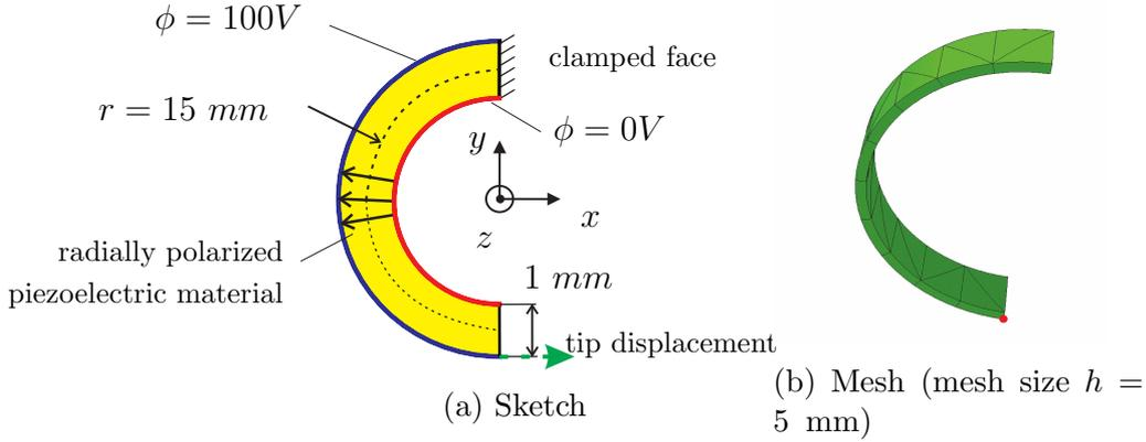
Figure 6: Sketch of radially polarized piezoelectric semicylinder and mesh used in *Netgen/NGSolve*
