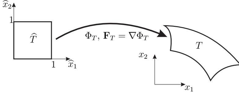
Figure 2: Transformation from unit element to deformed element
