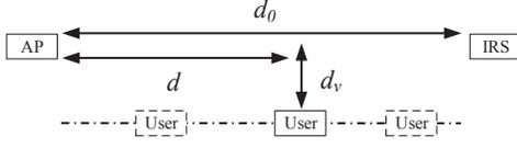
Fig. 2. Simulation setup.
