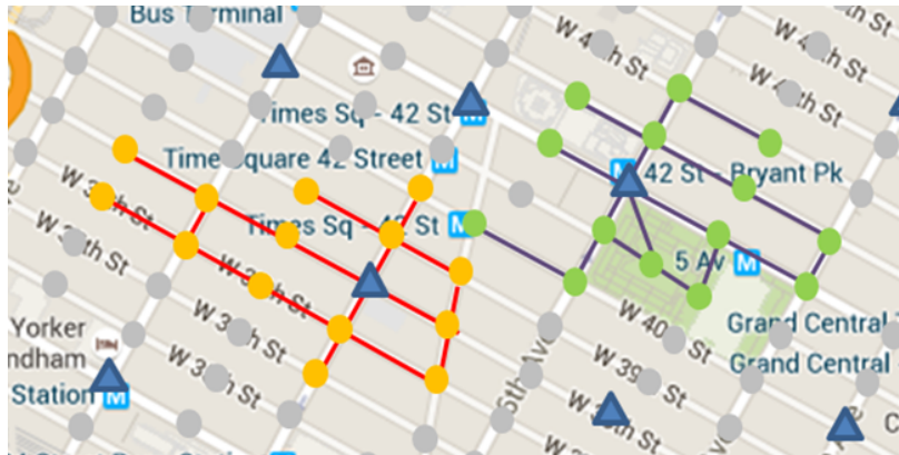
Figure 7: Example clusters formed by associating links to nearest gateway.
