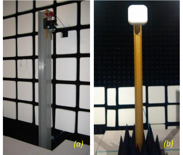
Fig. 1. NPL AC setup: (a) Transmitting tower with Tx ETS 3117 double-ridged horn antenna; (b) Receiving roll-over-azimuth positioner tower with the Laird PAS69278 MIMO AUT.
