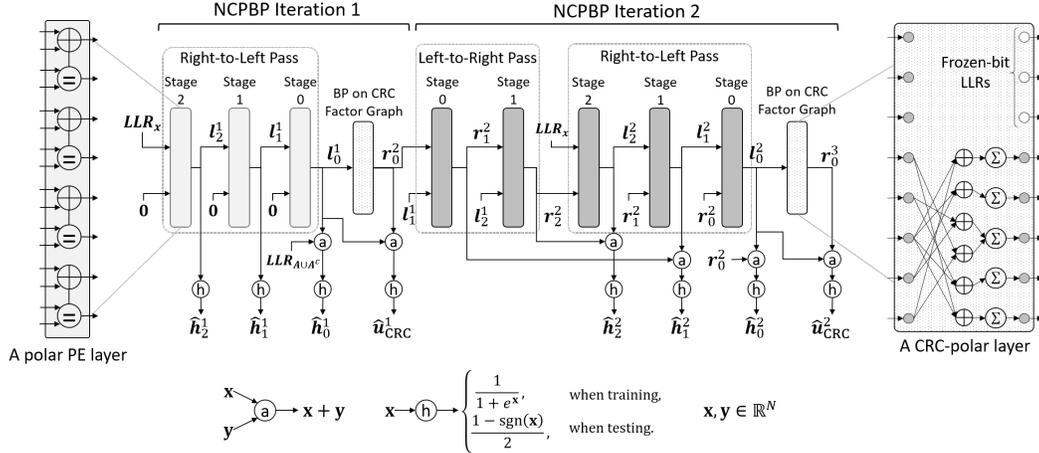
Fig. 5: NCPBP architecture with  $I_{\max} = 2$  and  $I_{\text{thr}} = 0$  for  $\mathcal{P}(8, 3)$  concatenated with a 2-bit CRC.
