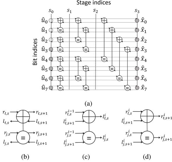
Fig. 1: (a) BP decoding on the factor graph of  $\mathcal{P}(8, 5)$  with  $\{u_0, u_1, u_2\} \in \mathcal{A}^c$ , (b) a PE, (c) a right-to-left message update of a PE on an unrolled factor graph, and (d) a left-to-right message update of a PE on an unrolled factor graph.
