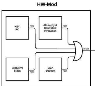
Figure 12: HW-Mod composition from sub-modules
