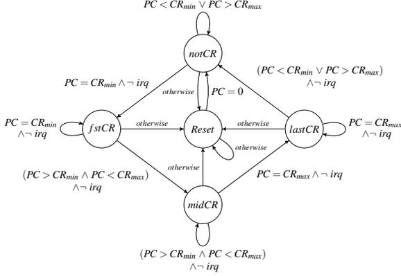
Figure 9: Verified FSM for atomicity and controlled invocation.
