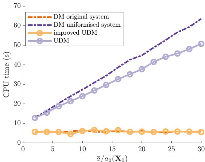
FIGURE 2. CPU time to generate  $N = 10^5$  sample paths with the UDM and improved UDM compared with the DM for different uniformisation rates  $\bar{a}$  relative to the initial total propensity  $a_0$ . Timings are for Example 4.3.1 with  $c_1 = 0.2$ ,  $c_2 = 0.1$  and  $\mathbf{X}_0 = (10, 0)$ , run until  $T = 10$ . Timing experiments were performed using MATLAB R2017b on an Ubuntu desktop PC with a 3.40 GHz Intel Core i7-2600K CPU and 16 GB of random access memory.
