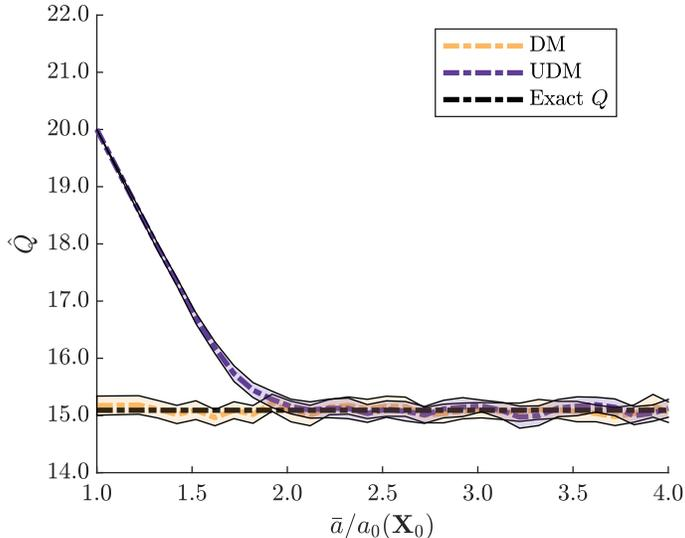
FIGURE 3. Bias effect due to invalid samples of the uniformised system for different uniformisation rates  $\bar{a}$  relative to the initial total propensity  $a_0$ . Model system used is Example 4.3.1 with  $c_1 = 0.4, c_2 = 0.1$  and  $\mathbf{X}_0 = (0, 20)$ , run until  $T = 10$ . The summary statistic is the number of  $X_1$  molecules at final time  $T$  and estimators are shown with 99.5% confidence interval for  $N = 10^3$  samples.
