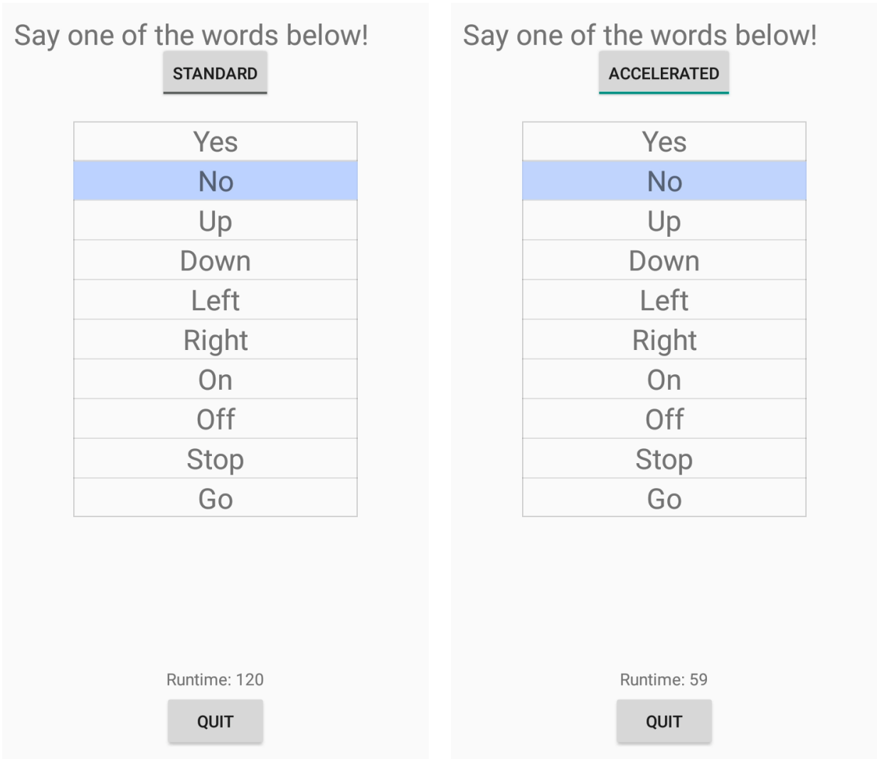
Figure 1: Recognition of a spoken word 'No' and runtimes (ms) on Android App. Left: full precision CNN model. Right: binary weight CNN model with 2x speedup.
