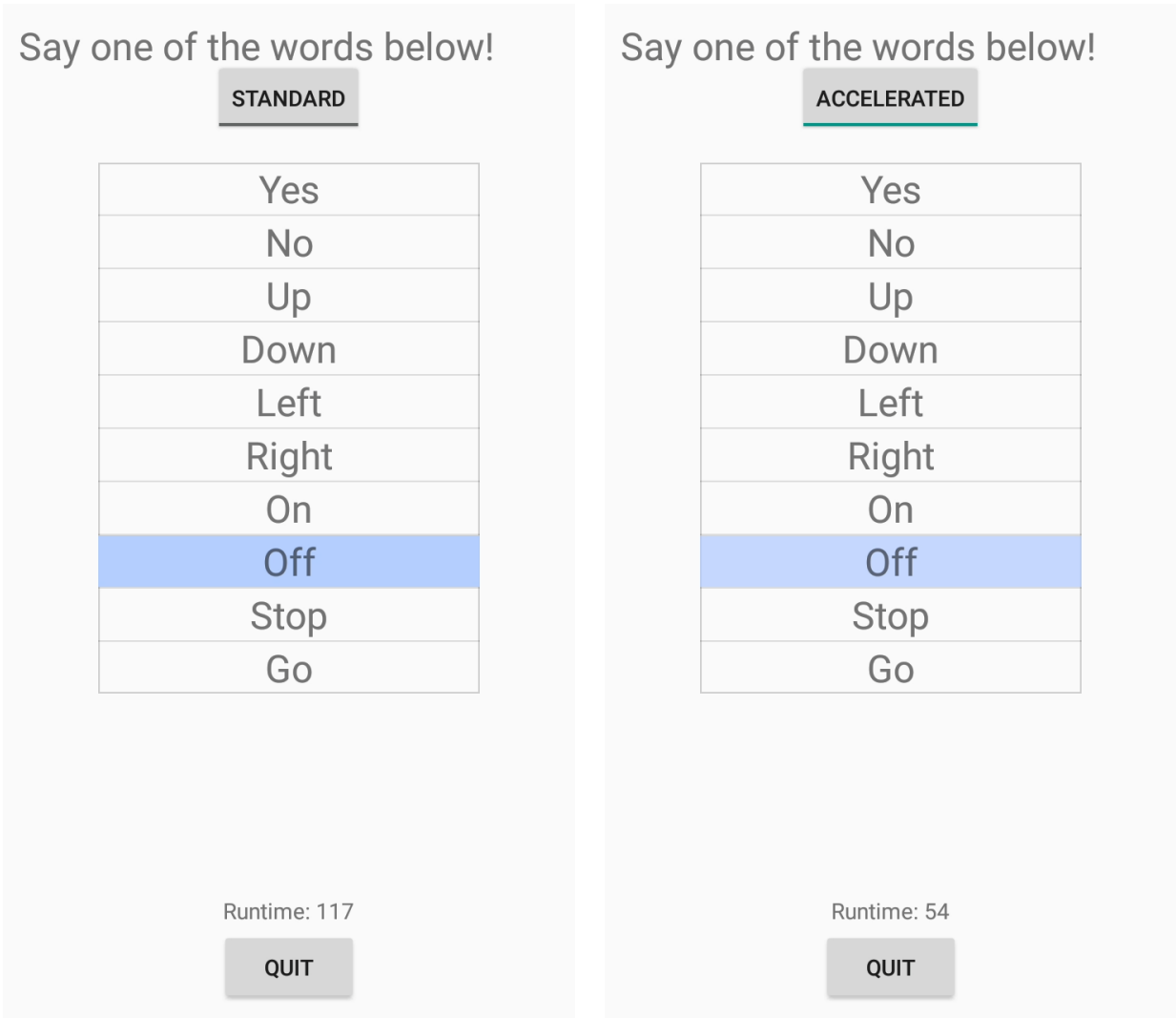
Figure 2: Recognition of a spoken word 'Off' and runtimes (ms) on Android App. Left: full precision CNN model. Right: binary weight CNN model with 2x speedup.
