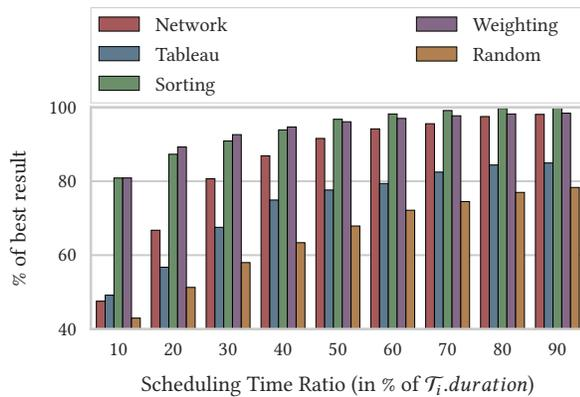
Figure 6: Relative performance under different time limits. Shorter scheduling times reduce the information for rewards and delay learning. The performance differences for Network and Tableau also arise from the initial exploration phase, as shown in Figure 5 (Data set: ABB Paint Control).
