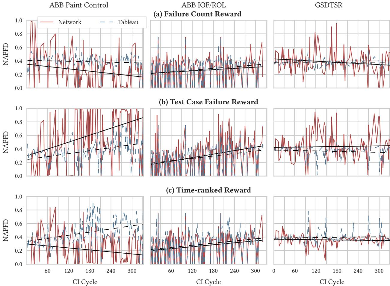
**Figure 4: Comparison of reward functions and memory representations: A Network-based agent with Test Case Failure reward delivers best performance on all three data sets (Black lines indicate trend over time)**
