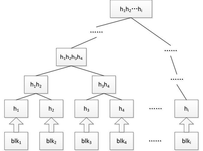
Fig. 3. The storage structure that can be used by a prover to reduce its computational complexity when generating proofs. Each leaf  $h_i$  stores the hash value of a block, and each internal node stores the product of the values stored at its two children.
