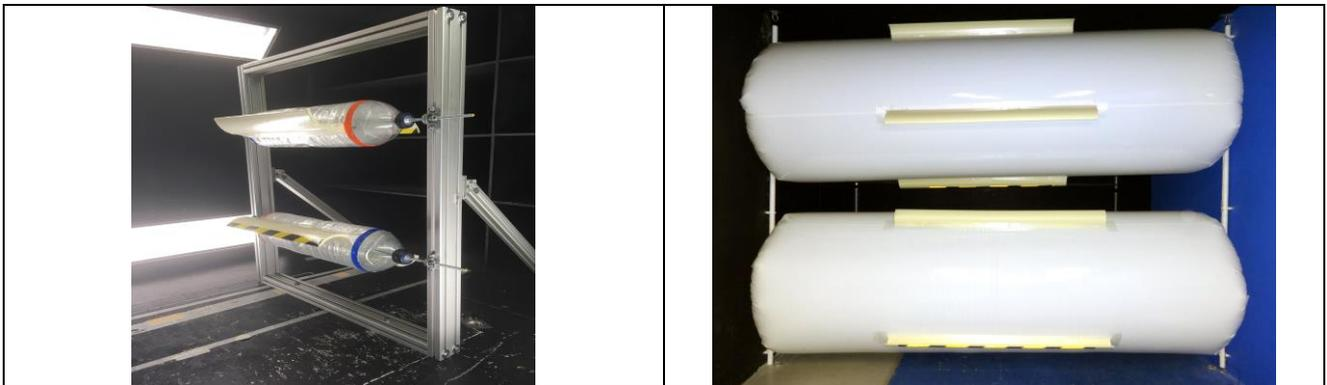
Figure 2: Experimental setups for novel aerostat wind turbine array testing.
