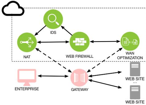
**Figure 7: System architecture of privacy preserving NFV platform used to process Web traffic**
