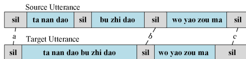
Fig. 2. Example of the aligned texts for a pair of parallel utterances. Texts are presented as Chinese pinyin and “sil” represents the silence. “a”, “b” and “c” represent totally three alignment points in this pair of parallel utterances. Therefore, totally C_3^2 (i.e., 3) potential parallel fragments can be sliced from original utterances.
