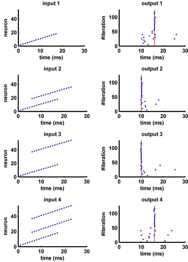
Figure 6: XOR problem: Input spike raster (left) and corresponding output spike raster (right - blue dots) obtained during NormAD based training of a  $54 \rightarrow 54 \rightarrow 1$  SNN with vertical red lines marking the position of desired spikes. The output spike raster is plotted for one in every 5 training iterations for clarity.
