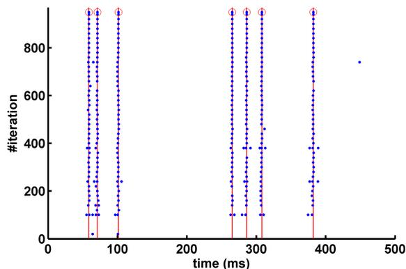
Figure 8: Illustrating NormAD based training of an exemplary problem for 3-layer  $100 \rightarrow 50 \rightarrow 25 \rightarrow 1$  SNN. The output spike rasters (blue dots) obtained during one in every 20 training iterations (for clarity) is shown, overlaid on plots of vertical red lines marking positions of the desired spikes.
