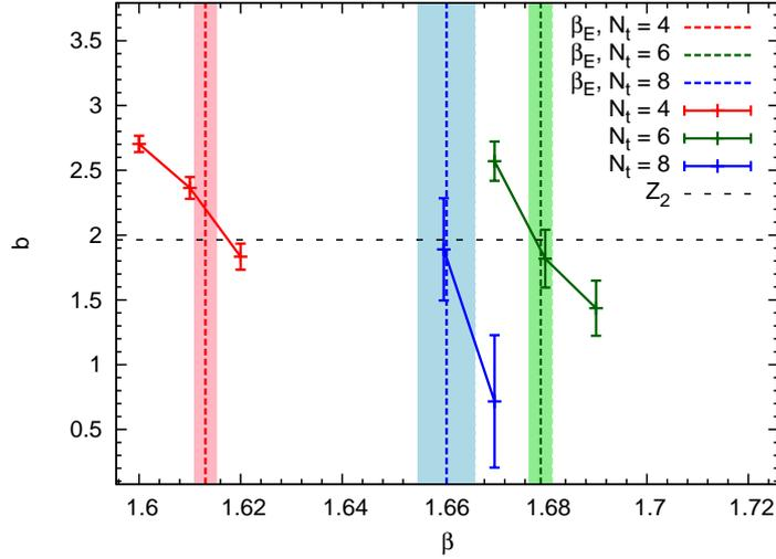
**Figure 3:**  $\beta$  dependence of the critical exponent  $b$  defined in Eq (3.2). Difference among colors means different  $N_t$ . Vertical dashed lines with bands indicate  $\beta$  values and their statistical errors at the critical endpoints for each  $N_t$ .  $b$  for the Z(2) universality class is also shown with a dashed horizontal line.
