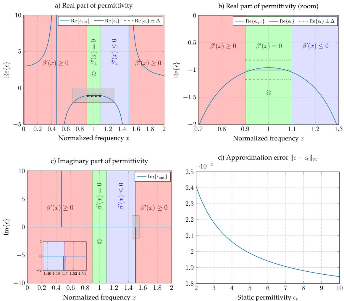
**Figure 5.** a-c) Real and imaginary parts of the optimal non-passive permittivity function approximating a metamaterial with  $\epsilon_t = -1$ ,  $\epsilon_s = 3$ , and  $\epsilon_\infty = 1$ . The zoomed-in region in a) is depicted in b). The corresponding sum-rule-bound limits based on (37) are given by  $\epsilon_t \pm \Delta$ ; d) Approximation error plotted as a function of the static permittivity  $\epsilon_s$ .
