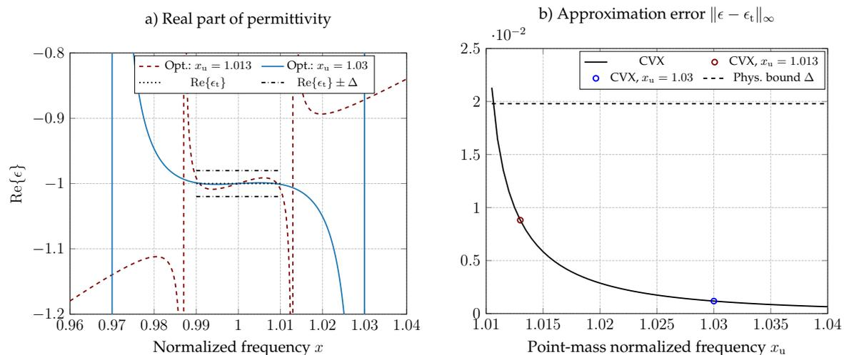
**Figure 4.** a) Real part of the non-passive permittivity function optimized with point masses only. The corresponding sum-rule-bound limits based on (37) are given by  $\epsilon_t \pm \Delta$ ; b) Approximation error as a function of upper point mass normalized frequency  $x_u$  (the normalized frequency of lower point mass is  $x_l = 1 - (x_u - 1)$ ).
