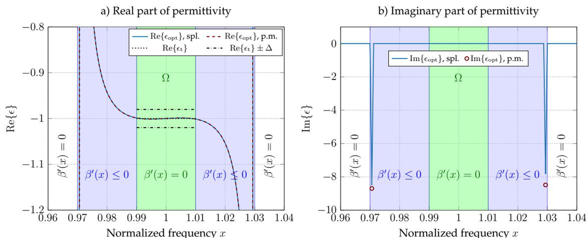
**Figure 2.** Real and imaginary parts of the optimal non-passive permittivity function approximating a metamaterial with given, negative target permittivity  $\epsilon_t = -1$  over the approximation domain  $\Omega$ . The corresponding sum-rule-bound limits based on (37) are given by  $\epsilon_t \pm \Delta$ . Two cases are considered, a spline approximation in  $I_2$  (blue) and the point mass approximation in  $I_2$  (dark-red).
