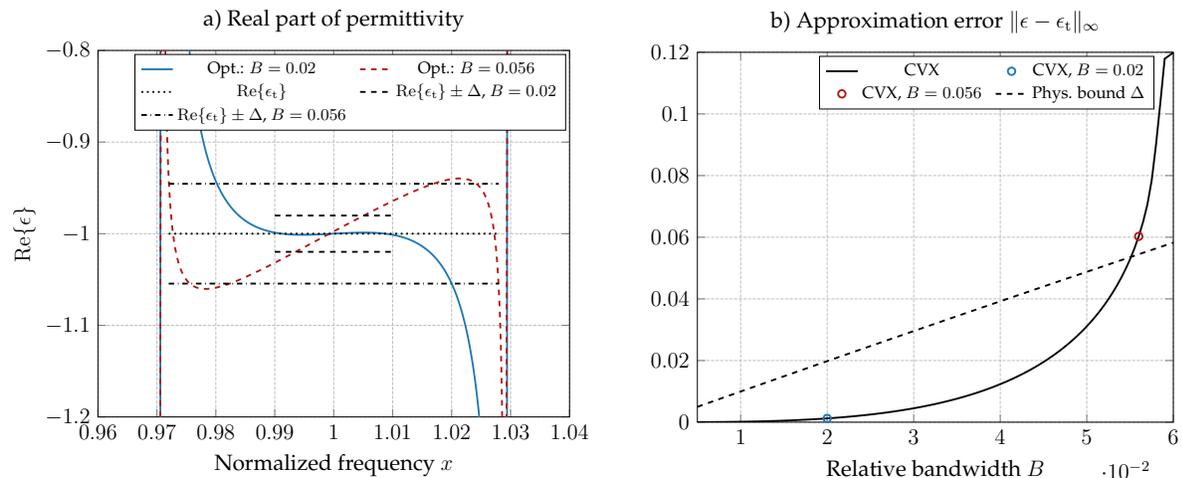
**Figure 3.** a) Real part of the non-passive permittivity function approximating a metamaterial with given  $\epsilon_t = -1$  over the approximation domain  $\Omega = [1-B/2, 1+B/2]$ ; b) Approximation error as a function of relative bandwidth  $B$ .
