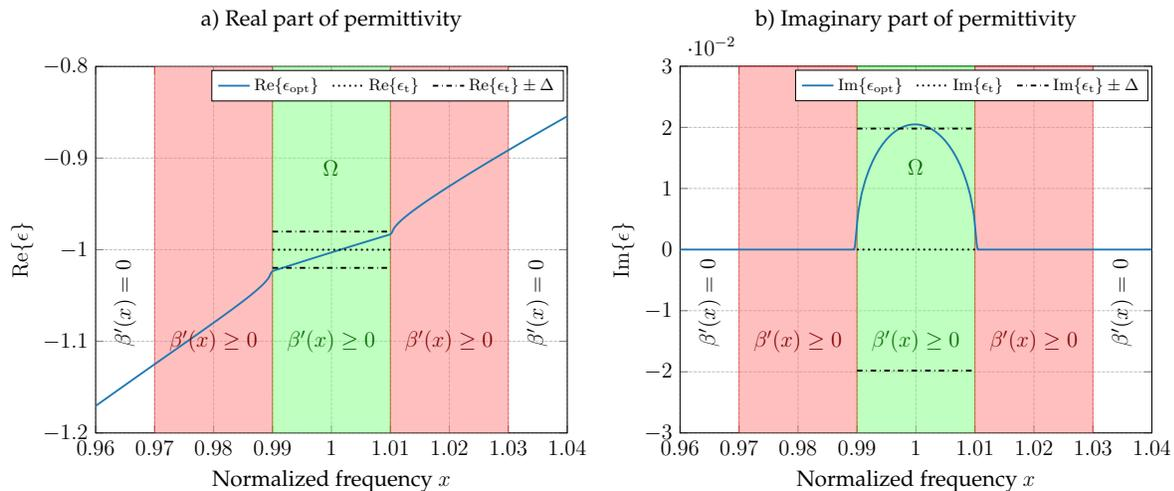
**Figure 1.** Real and imaginary part of the optimal passive permittivity function approximating a metamaterial with given  $\epsilon_t = -1$  over the approximation domain  $\Omega$ . The corresponding sum-rule-bound limits based on (37) are given by  $\epsilon_t \pm \Delta$ .
