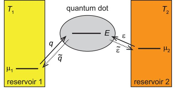
FIG. 2. (Color online) Schematic of the model. There are two reservoirs or leads 1 and 2 with temperatures  $T_1$  and  $T_2$  and chemical potentials  $\mu_1$  and  $\mu_2$ , respectively. Electron can move from one reservoir to the other via the quantum dot which has a well-defined single energy level  $E$ . The transition rate from the reservoir 1 (2) to the dot is  $q$  ( $\epsilon$ ) and the reversed rate is  $\tilde{q}$  ( $\tilde{\epsilon}$ ).
