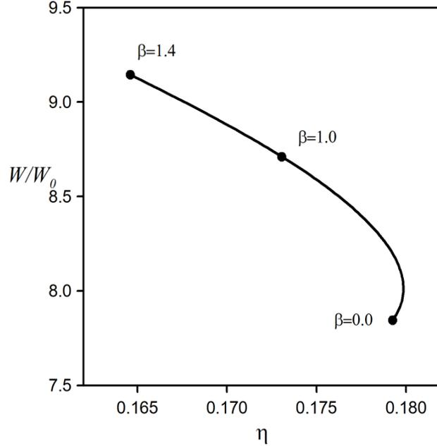
FIG. 4: Dimensionless work as a function of the efficiency when the polytropic index  $\beta$  varies between 0.0 and 1.4. The dots on the curve indicate three particular values of  $\beta$ . The other parameters are the same as those of previous figures.
