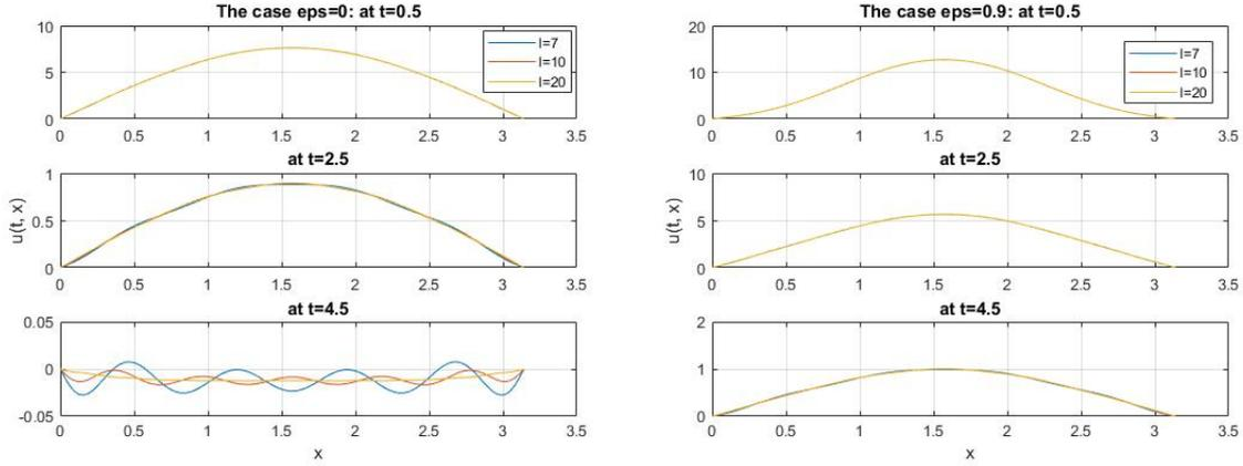
FIGURE 2. In the plots we illustrate the graphics of the solution  $u$  of the inverse problem (7.1)–(7.4) for parameters  $\varepsilon = 0$  and  $\varepsilon = 0.9$  at  $t = 0.5, 2.5, 4.5$ . Here the graphics of  $f$  are given for different  $l = 7, 10, 20$ , and colored in blue, red, yellow, respectively.
