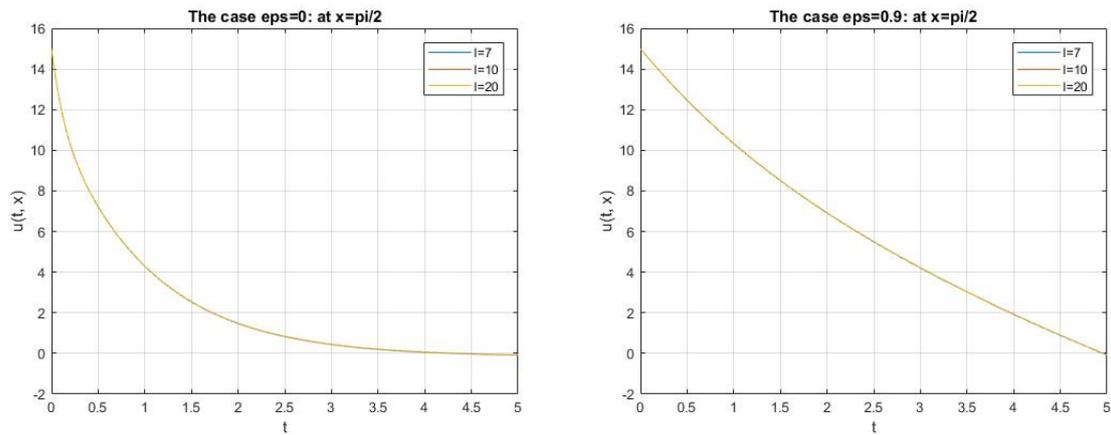
FIGURE 4. In the plots the graphics of the solution  $u$  of the inverse problem (7.1)–(7.4) are shown at  $x = \pi/2$  in the cases  $\varepsilon = 0$  and  $\varepsilon = 0.9$ . Here the graphics of  $f$  are given for different  $l = 7, 10, 20$ , and colored in blue, red, yellow, respectively.
