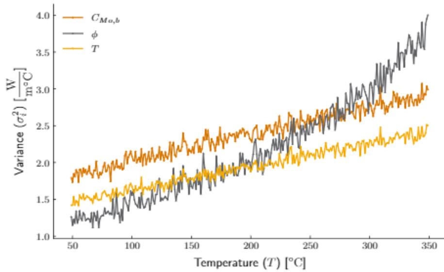
Figure 5: Results of univariate sensitivity analysis of several important input variables (concentration of Mo at BOL,  $C_{Mo,b}$ , neutron flux,  $\Phi$ , and average ATR loop temperature,  $T$ ) and their calculated temperature dependent effect on the output thermal conductivity in units of W/m °C.
