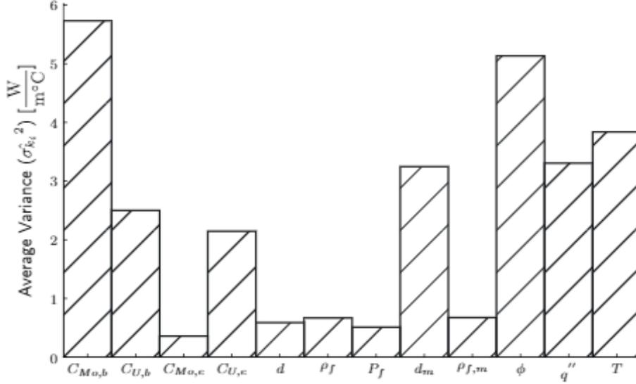
Figure 4: Results of univariate sensitivity analysis of each input variable and its absolute effect on the output thermal conductivity in units of  $W/m \cdot ^\circ C$ . The variance plotted above for each input variable is averaged over the temperature range of 0 to  $350^\circ C$ .
