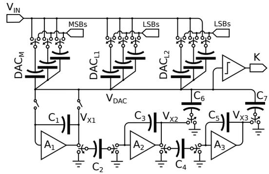
Fig. 5. Implementation of the capacitor network used to perform signal conversion using the bottom sampled capacitor arrays  $DAC_M$  for the DWA bits and  $DAC_{L1}$  &  $DAC_{L2}$  for the MES bits. The loop filter is also shown where  $A_1$  amplifies the quantisation residue that is then integrated by  $A_2$  &  $A_3$  for noise-shaping.
