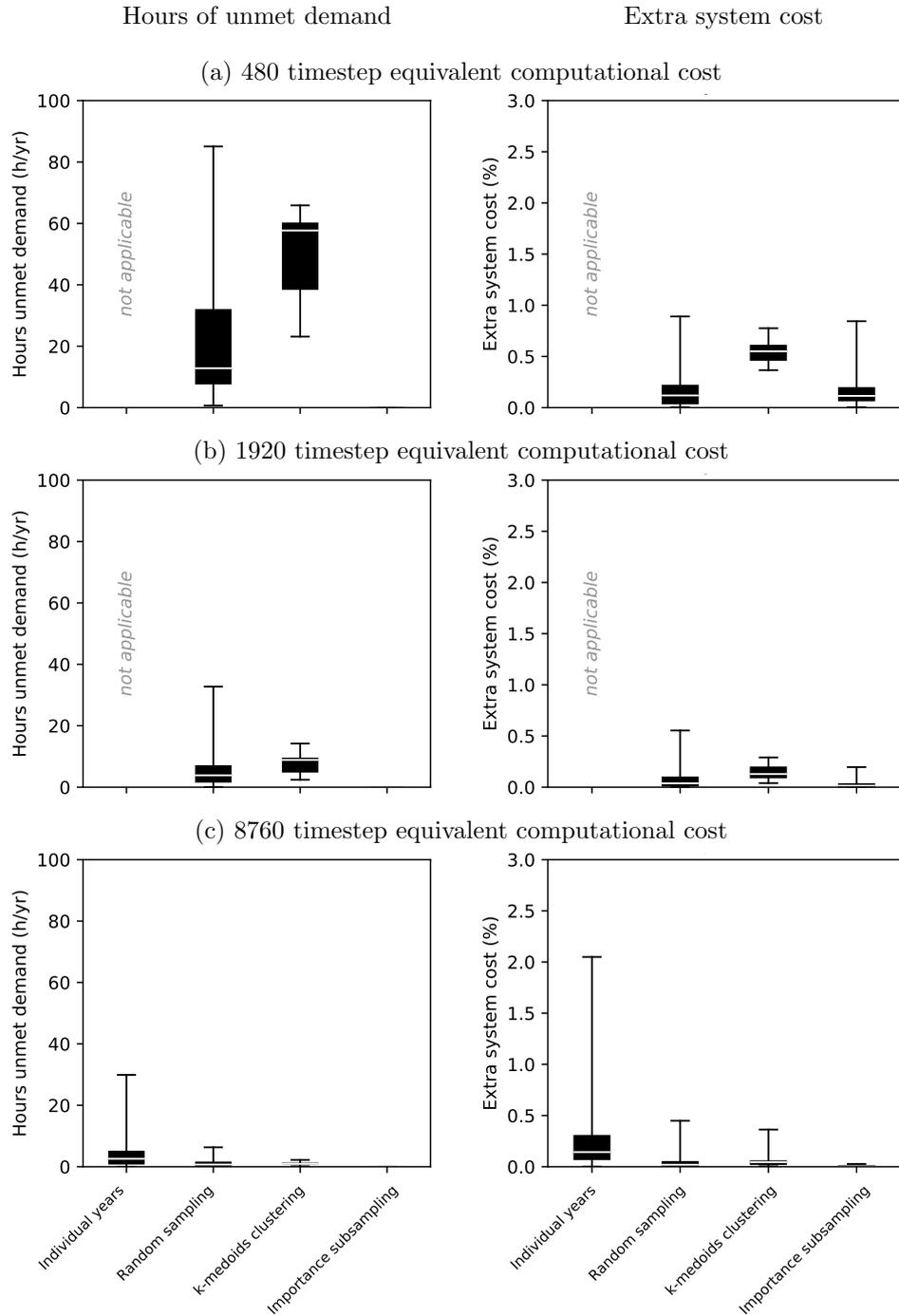
Figure 5: Distribution of *hours of unmet demand* and *extra system cost* for different subsampling methodologies. The box shows the 25th, 50th (median) and 75th percentiles, while the whiskers show the 2.5th and 97.5th. (a) corresponds to a computational cost equivalent to a single PSM run using 480 timesteps, while (b) and (c) correspond to 1920 and 8760 timesteps respectively and the target under subampling.
