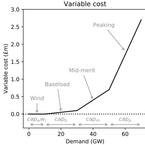
Figure 3: A timesteps’s variable cost as a function of demand. The first  $\text{cap}_w w_t$  (installed wind capacity times wind capacity factor) GW are met by wind (with no contribution to variable cost), followed by baseload, mid-merit and peaking. The variable cost increases more quickly as progressively more expensive generation technologies are employed.
